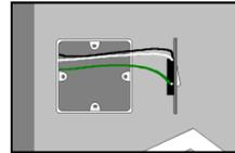
4. Use fixing screws provided to fix switch assembly onto wall box. Tighten screws evenly a little at a time until just tight enough to prevent movement of the back plate. Do not over-tighten screws as this will deform the plastic clip on the switch assembly, inhibiting the faceplate from being securely fixed.
