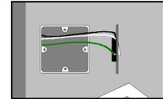
4. Use fixing screws provided to fix switch assembly onto wall box. Tighten screws evenly a little at a time until just tight enough to prevent movement of the back plate. Do not over-tighten screws as this will deform the plastic clip on the switch assembly, inhibiting the faceplate from being securely fixed.
