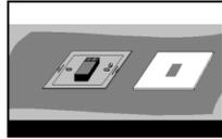
2. Ensure wall is flat around wall box removing any lumps of plaster and sanding away any uneven plaster.
