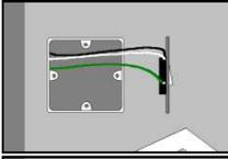
4. Use fixing screws provided to fix switch assembly onto wall box. Tighten screws evenly a little at a time until just tight enough to prevent movement of the back plate. Do not over-tighten screws as this will deform the plastic clip on the switch assembly, inhibiting the faceplate from being securely fixed.
