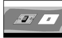
2. Ensure wall is flat around wall box removing any lumps of plaster and sanding away any uneven plaster.
