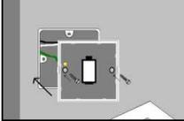
5. Pick up decorative front plate carefully and push into place, pressing gently on each side to ensure the front plate has engaged with the plastic clips on the switch assembly.
