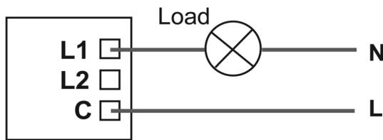
**Figure 1.** Using a 1-Way Dimmerswitch
