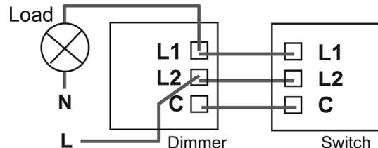
**Figure 4.** Using a 2-Way Dimmerswitch
