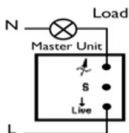
Fig 1. Wiring for 1-Way Circuits
