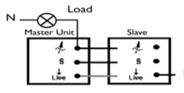
Fig 3. Alternative Wiring for Multi-Way Circuits
