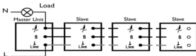
Fig 2. Wiring for Multi-Way Circuits
