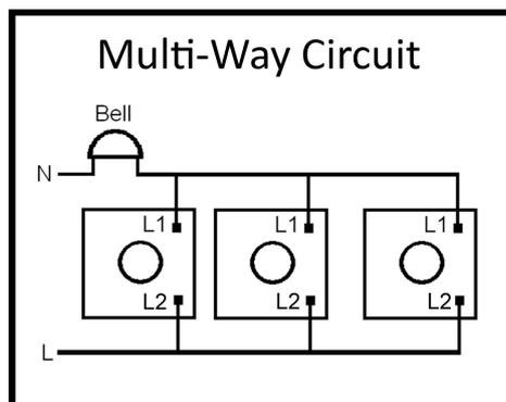
**WARNING:** The switches in these products are rated at 6 or 10A (Please check the rear of the product for rating). Check the in-rush current for LED bulbs or drivers does not exceed 6 or 10A before connecting. Fit inrush current limiters where necessary.
