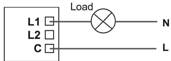
**Figure 2.** Using a 1 or 2-Way Dimmerswitch
