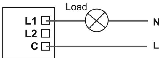
**Figure 1.** Using a 1-Way Dimmerswitch
